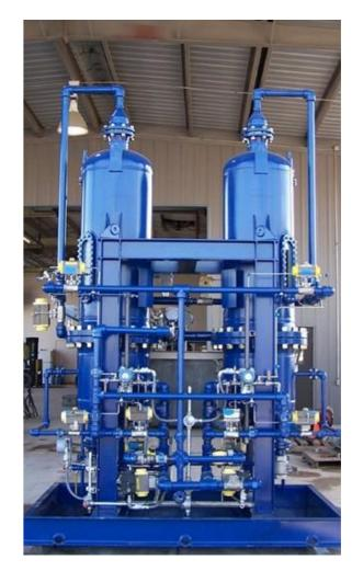
The filter operates at twice the flux rate of conventional sand filters in the same application, and can remove over three times the amount of solids before needing to be cleaned.
